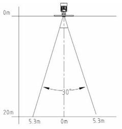
DN100 Horn antenna beam angle
