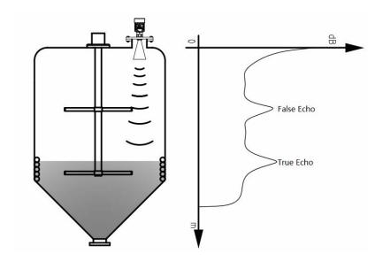
As the following figure shows, we can save the false echoes between the envelope curves, and obtain the level echo.
