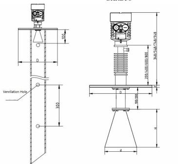
Note: Flange Dimensions refer to flange specification Horn dimensions refer to horn specification
