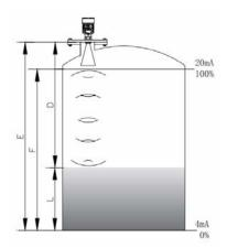
▶ Input: The antenna receives the reflected microwave impulse and transmits it to the electric circuit, the micro processor processes this signal, recognizes the wave echo produced by microwave impulse on the substance surface. The correct microwave echo signal recognition is completed intelligent software, the precision can reach millimeter grade. The distance from the substance surface D is proportional to impulse time stroke T:  $D=C \times T/2$  ( C is velocity of light)
