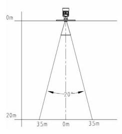
DN150 Horn antenna beam angle
