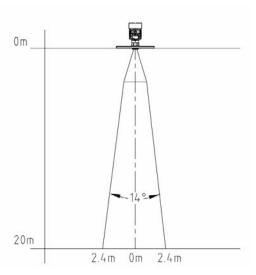
DN250 Horn antenna beam angle
